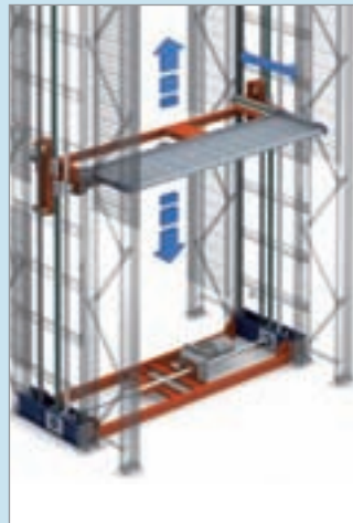
Extractor-elevator drive operation
